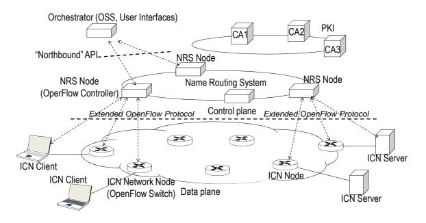
Figure 3- Information Centric Network based on extended OpenFlow
