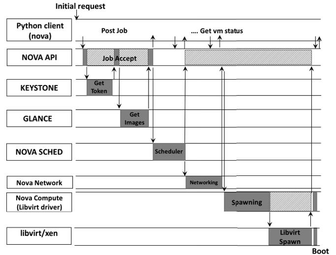
Fig. 4. VIM instantiation model for OpenStack Nova
