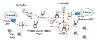
Fig. 3. Controller selection by a Wireless Mesh Router
