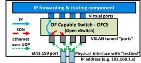
Figure 5. Implementing VXLAN tunnels using Open vSwitch (OVS)
