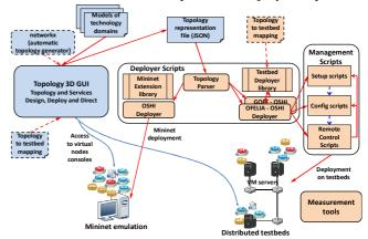
Figure 2. Mantoo enabled emulation workflow
