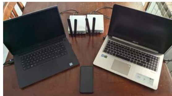
Figure 6: LTE IMSI Catcher experimental setup.
